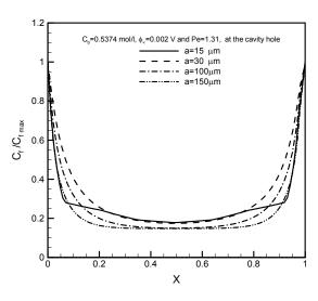
Fig. 8. Friction coefficient ratio  $C_f$  /  $C_{f_{\rm max}}$  versus X for  $C_b$ = 0.5374 mol/l,  $\phi_{\infty}$ =0.002 V, Pe=1.31 and various a=15~150  $\mu$ m.
