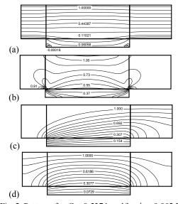
Fig. 2. Patterns for  $C_b$ = 0.5374 mol/l,  $\phi_{\infty}$  =0.002 V, a=100  $\mu$ m and Pe=1.31, (a) Streamline (b) Isostrain-rate (c) Isoconcentration (d) Isovoltage.
