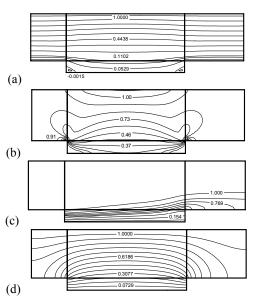
Fig. 3. Patterns for  $C_b$ = 0.5374 mol/l,  $\phi_{\infty}$  =0.002 V, a=100  $\mu$ m and Pe=41.6, (a) Streamline (b) Isostrain-rate (c) Isoconcentration (d) Isovoltage.
