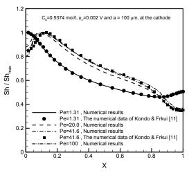
Fig. 6. Mass fraction  $Sh/Sh_{\rm max}$  versus X for  $C_b$ = 0.5374 mol/l,  $\phi_{\infty}$ =0.002 V, a=100  $\mu$ m and various Pe=1.31 $\sim$ 100.
