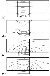
Fig. 4. Patterns for  $C_b$ = 0.5374 mol/l,  $\phi_{\infty}$  =0.002 V, Pe=1.31 and a=30  $\mu$ m, (a) Streamline (b) Isostrain-rate (c) Isoconcentration
