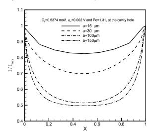
Fig. 9. Current density fraction  $I/I_{\rm max}$  versus X for  $C_b=$  0.5374 mol/l,  $\phi_{\infty}$  =0.002 V, Pe=1.31 and various a=15~150  $\mu$ m.
