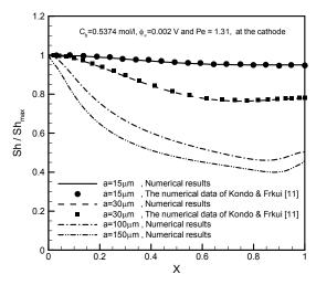
Fig. 7. Mass fraction  $Sh/Sh_{\rm max}$  versus X for  $C_b$ = 0.5374 mol/l,  $\phi_{\infty}$  =0.002 V, Pe=1.31 and various a=15 $\sim$  150  $\mu$ m.
