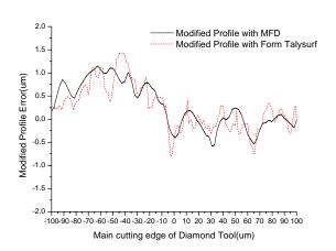
Fig.6. Comparison between the MFD-generated profile and profile measured by Form Talysurf.
