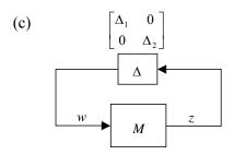
Fig.1. (a) Closed-loop demanding for robust performance, (b) Robust stability of Figure 1a, (c) Fractional transformation of Figure 1b.
