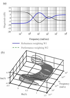
Fig.4. (a) Robustness and performance weightings of Example 2, (b) The  $\mu$  -manifold of Example2.
