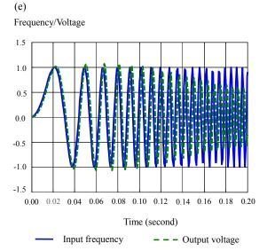
Fig.8. (d) Reliability distance of the chosen loop, (e)A pilot run of the frequency-to-voltage transducer.
