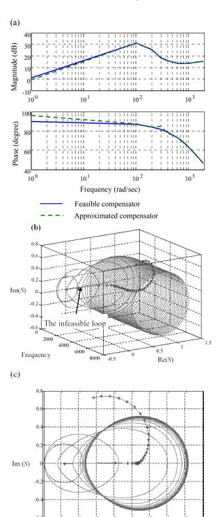
Fig.9. (a) The compensator pertaining to maximum reliability distance, (b) The sensitiveness of high-order system to fast-timed operation, (c) The projected view of Figure 9b.
