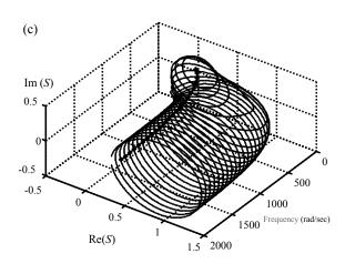
Fig.8. (a) The  $\mu$ -manifold in magnitude-phase coordinate, (b) To find a feasible loop in the  $\mu$ -manifold, (c) The chosen loop inside  $\mu$ -manifold.
