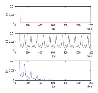
Fig. 1. Norm of error in magnified scale by (a) sign-type (b) saturation-type and (c) improved SMC designs.
