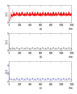
Fig. 2. Norm of control effort by (a) sign-type (b) saturation-type and (b) improved SMC designs.
