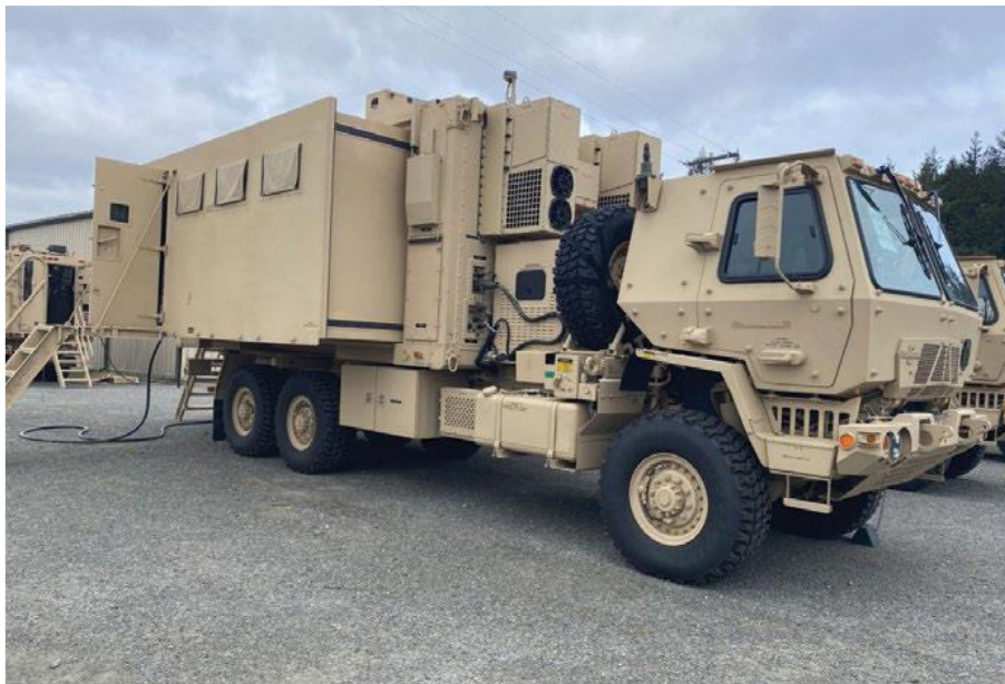
An M1087 Expandable Van Shelter houses the Command Post Integrated Infrastructure System under operational test (Photo by Sgt. 1st Class Frederick E. Estep, U.S. Army Operational Test Command)
