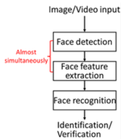
Fig. 1. A procedure of a computer-based face recognition (Source: [3])
