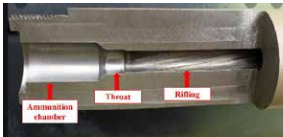
Fig.1. Main Structure of a gun barrel
