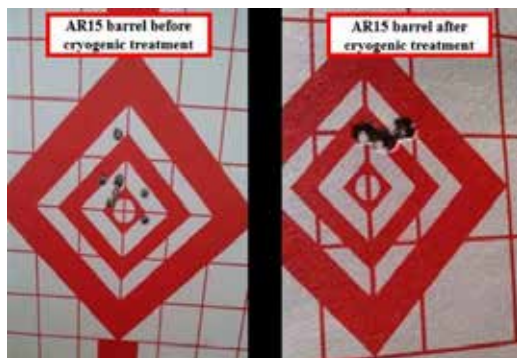
Fig.3. Shooting results of the AR15 barrel before/ after cryogenic treatment [14]
