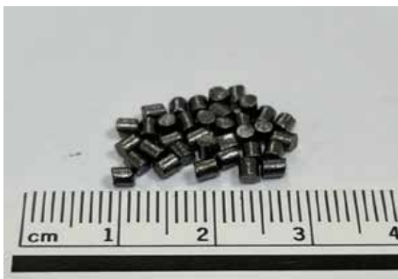
Fig.1. The sample of nitramine gun propellant of unknown composition from the arsenal in Taiwan
