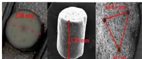
Fig.3. Detailed geometric information of the gun propellant sample.
