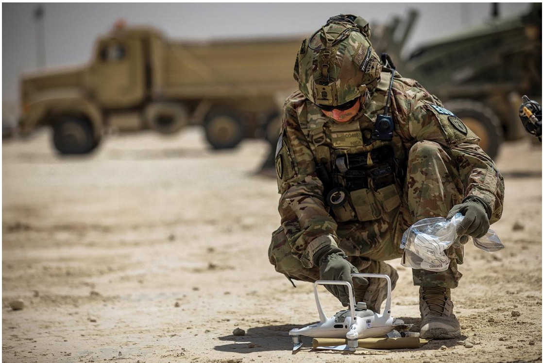
Sgt. 1st Class Adrian Coghill, an explosive ordnance disposal technician, sets up a remote-controlled ordnance disposal drone at the Ain al-Asad air base, Iraq. (Credit: U.S. Army/Spc. Derek Mustard)
