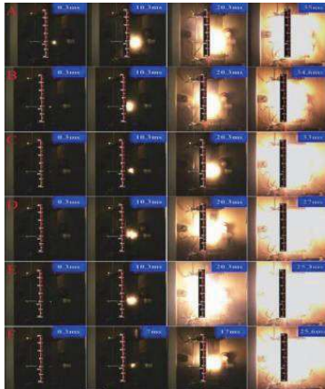
Fig. 9. Snapshots of flame propagation of dust explosion for Ti powder with an average particle size of 35 nm [Dust weight: (A) 300, (B) 600, (C) 900, (D) 1200, (E) 1500, and (F) 1800 mg; Ignition energy: 1 mJ]
