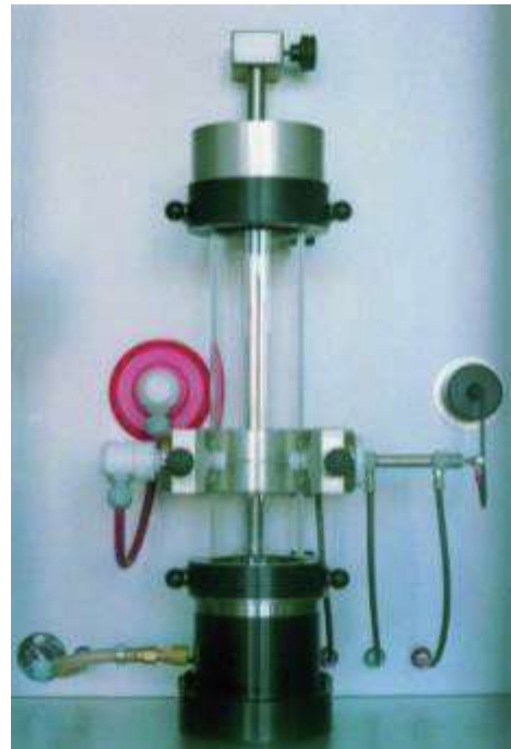
Fig. 3. Photo of modified Hartmann tube (Manual for modified Hartmann tube)
