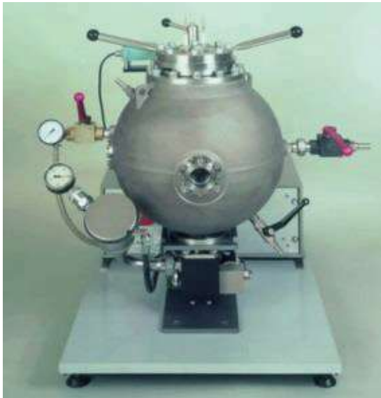
Fig. 2. Photo of 20-L explosion sphere apparatus (Manual for 20-l-Apparatus)
