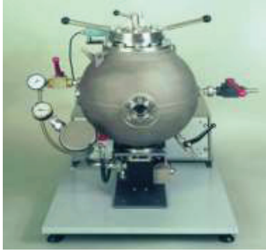
Fig. 2. Photo of 20-L explosion sphere apparatus
