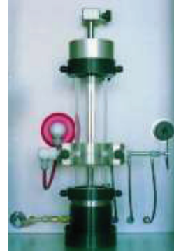
Fig. 3. Photo of modified Hartmann tube
