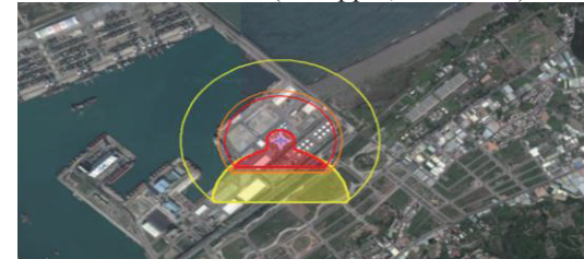
Fig 5. The hazard range from inflammable vapor cloud in annual wind situation
