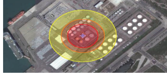
Fig 3. The hazard range of thermal radiation from pool fire in annual wind situation
