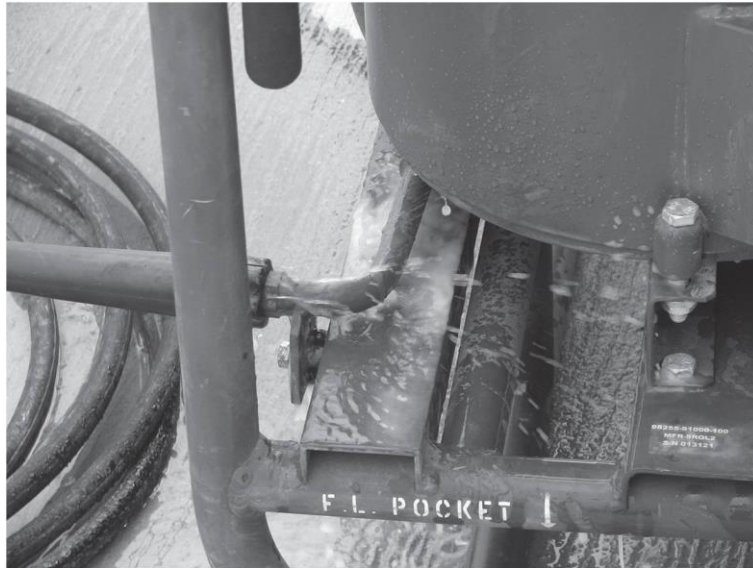
Figure 5. M26 decontamination apparatus O-ring failure
