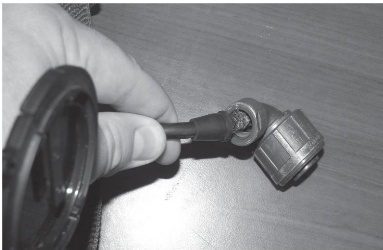
Figure 8. AN/PDR-75 cable damage from separation
