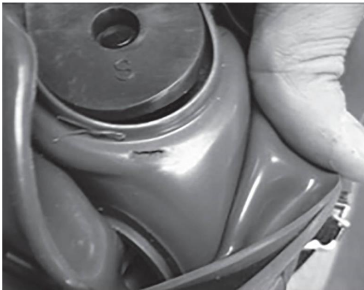
Figure 2. M40 series protective mask with a torn face blank
