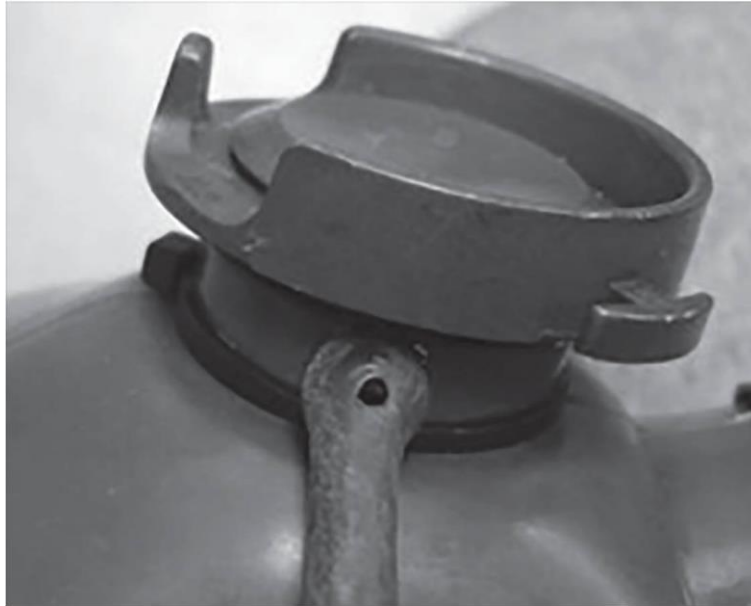
Figure 3. Torn M40 series protective mask external drink tube
