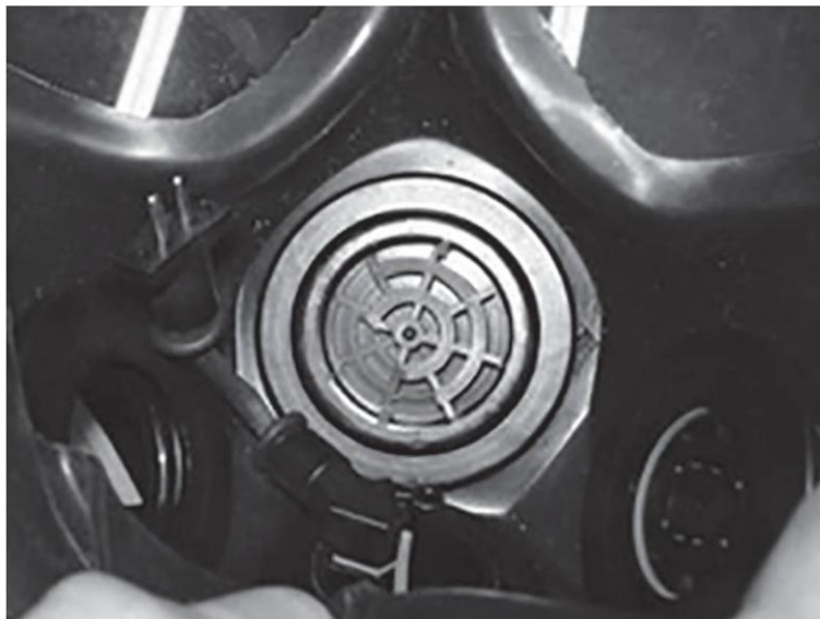
Figure 4. Damage to the front of the voicemitter on a M45 protective mask
