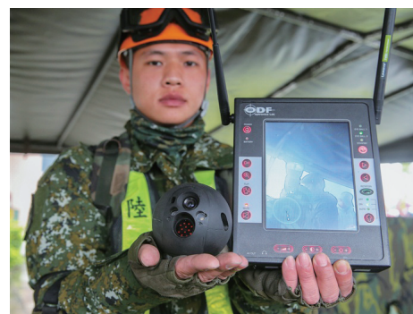
“Search Ball” is a wireless remote-controlled camera that shoots 360-degree images to locate survivors buried under collapsed structures. (Source: Military News Agency)
