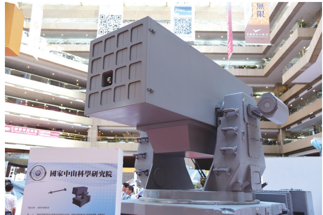
The Sea Oryx is an efficient system to intercept incoming anti-ship missiles and aircraft. (Source: Military Link Magazine)
