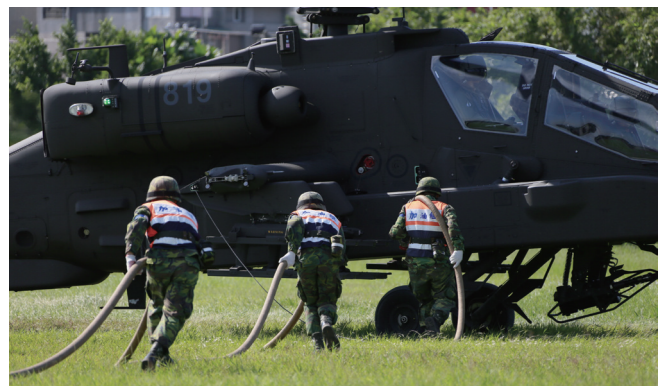
ROCA work crews perform an emergency refueling for an AH-64E with its engine still on. (Source: Military News Agency)
