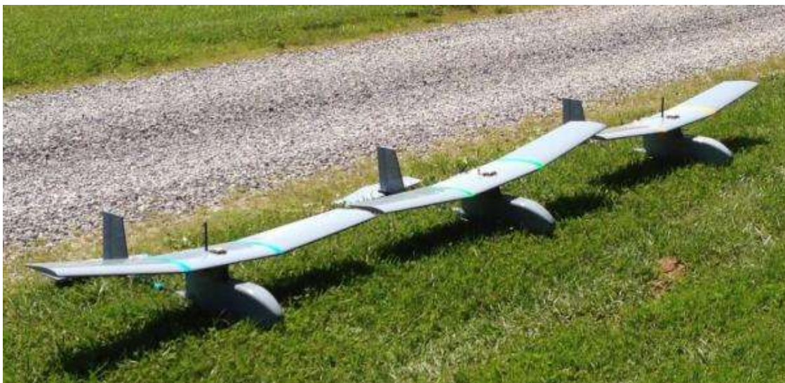
Figure 5: Model Planes Used as Surrogate for Raven RQ-11.
