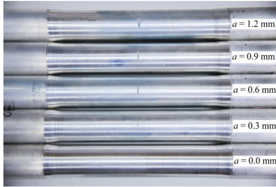
Fig. 6 A picture a local sharp-cut 6061-T6 aluminum alloy tube with D_o/t = 16.5 and a = 0.0, 0.3, 0.6, 0.9 and 1.2 mm
