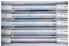
Fig. 6 A picture a local sharp-cut 6061-T6 aluminum alloy tube with  $D_0/t = 16.5$  and a = 0.0, 0.3, 0.6, 0.9 and 1.2 mm
