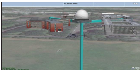
Fig.21 The radar station was designed among several buildings to test the impact of buildings on the radar's ability to detect
