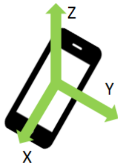
Figure 6. Motion of the tri-axis accelerometer in a smart phone when a user is walking
