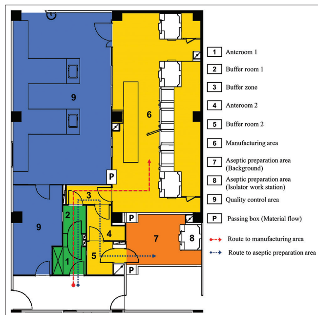
Figure 1: The redesigned clean rooms and the personnel flow. The reconstructions featured clear separation between different work areas and resulted in routes designed according to the principles of good manufacturing practice to keep off the cross-contamination. Furthermore, we set the environmental sensors to monitor the temperature, humidity, and pressure in each section. Information was recorded by Web-Based Building Automation system (WebCTRL®)
