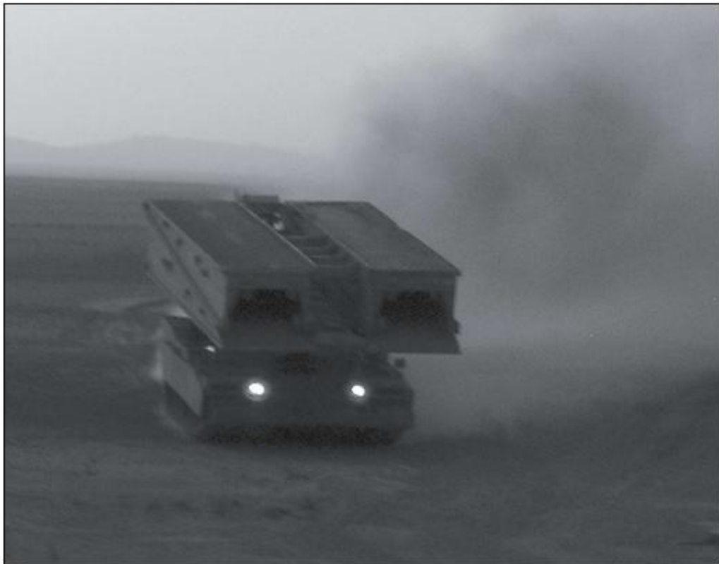
The Wolverine, with the HAB in place, maneuvers to the bridging site.
