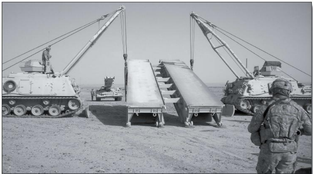
Operators use armored recovery vehicles to suspend the HAB in preparation for attachment to the Wolverine in the background.
