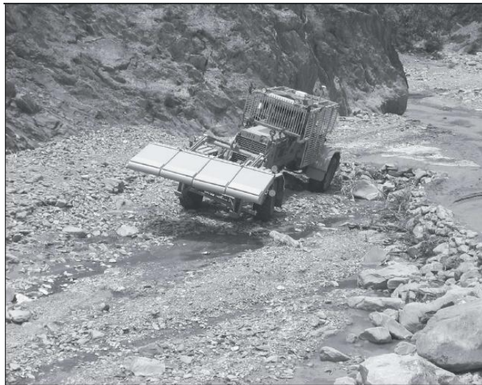
A Husky mounted detection system performs route clearance. 賀斯基排雷系統執行道路清除。
