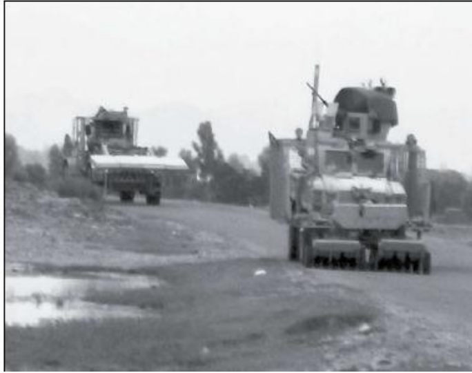
A mine-resistant, ambush-protected vehicle with mine rollers and a Husky mounted mine detection vehicle participate in route clearance operations in Khowst Province, Afghanistan. 一輛防地雷突擊車(MRAP)、排雷犁與賀斯基地雷裝載與偵測車(HMDs)在阿富汗霍斯特(Khowst)省執行道路清除任務。
