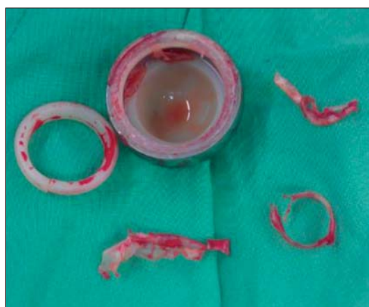
Figure 3. The removed prosthesis showed broken locking ring (the arrow pointed the broken area) and the worn polyethylene insert in the inferior rim (asterisk). There still were some small pieces of polyethylene debris in the hip joint
