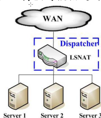
圖四 LSNAT 運作架構圖(資料來源:Gan, D. and Srisuresh, P., “Load Sharing using IP Network Address Translation(LSNAT)”, RFC2391,1998.)
