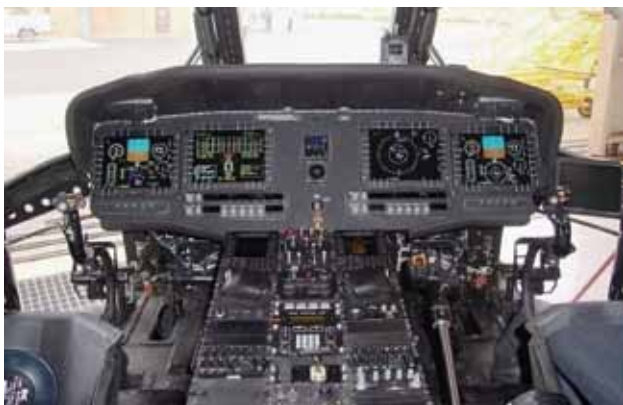
HH-60M的全數位化駕駛艙，艙內下方的對外視野極佳。(照片來源：Sikorsky S-70A，Jane's All the World's Aircraft，February 15, 2012)
