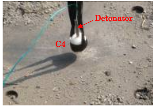
Fig. 3 M6 detonator connected to C4 explosive
