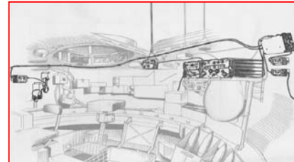
圖 17：M41 戰車無線電機配置 (The reference source : Rebuilding form network's pictures)
