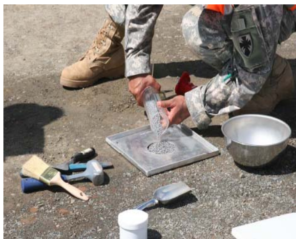
圖 15：為 JRAC 專案進行鋼珠密度試驗實景 參考資料：Travis A. Mann, JOINT RAPID AIRFIELD CONSTRUCTION TECHNOLOGY DEMONSTRATION, Engineer Research and Development Center, USACE,2009,p10.
