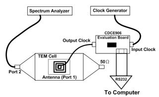
Fig.1. Experiment setup for measuring the RE of the spiral antenna excited by the CDCE906 output clock.
