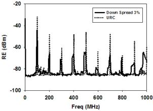
Fig.2. Radiated emissions from the antenna excited by the down-spread SSC with  $\delta = 3\%$  and the corresponding URC (or SSC with  $\delta = 0$ );  $f_c = 100$  MHz.
