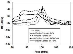
Fig.3. RE of spread SSCs with two different spreading schemes and with or without a 3 ns longer rise/fall time at fundamental frequency 100 MHz.
