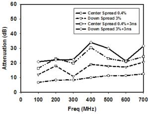
Fig.4. Attenuation values of the  $\delta = 3\%$  down-spread and the  $\delta = \pm 0.4\%$  center-spread schemes, both with and without an additional rise/fall time of 3 ns;  $f_c = 100$  MHz.
