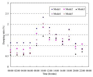
Fig.6. Variation of damping ratios identified with time of day in torsional direction
