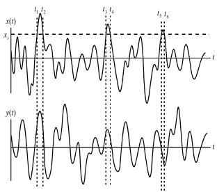
Fig. 3. Construction of Randomdec signatures [19].
