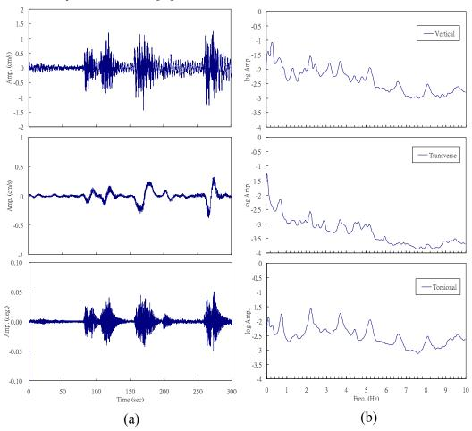
Fig. 2. Typical set of recorded data from monitoring system with corresponding auto- spectra in the three directions. (a) Time history, and (b) corresponding auto-spectra.
