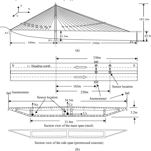
Fig.1. Layout of the Kao Ping Hsi cable-stayed bridge: (a) plane view; (b) sensor locations of the structural monitoring system.
