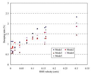
Fig.8. Variation of damping ratios identified vs RMS velocity in torsional direction (at 1/2 of main
