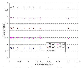
Fig.7. Variation of frequencies identified vs RMS velocity in torsional direction
