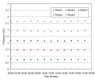
Fig.5. Variation of frequencies identified with time of day in torsional direction
