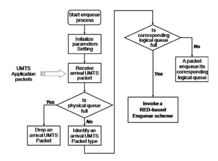
Fig. 3. The flowchart of the two-stage enqueuing process.
