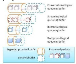
Fig. 1. A diagram of the dynamic queue buffer allocation.
