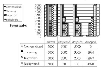
Fig. 6. Simulation results of all UMTS traffic in a continuous transmission pattern.
