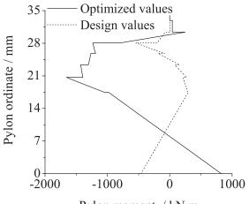
$Pylon\ moment\ /\ kN\cdot m$  Fig.9. Comparison of pylon moments.
