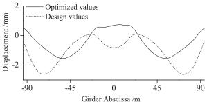
Fig.8. Comparison of girder displacements.
