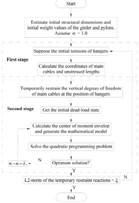
Fig.4. Flow chart for the two-stage approach method.
