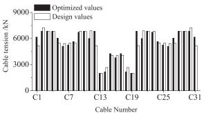
Fig.6. Comparison of cable tensions.
