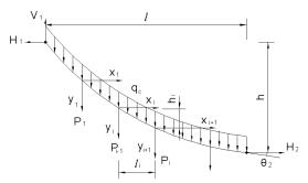
Fig. 3. Mechanical diagrammatic sketch of the main cable.
