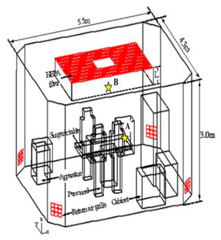
Fig. 2. Geometric model of the operation room.
